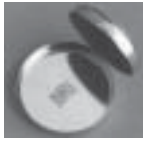
Silicon memory chip inside the ibutton™.
